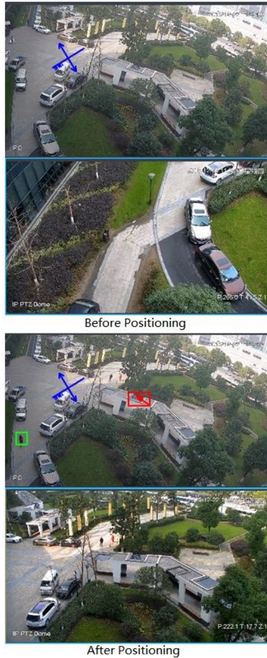
Figure 3-166 3D positioning (Zoom out after positioning)
